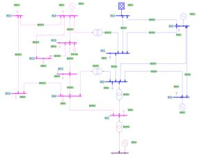
Fig. 3: One-line diagram of IEEE 14 system
